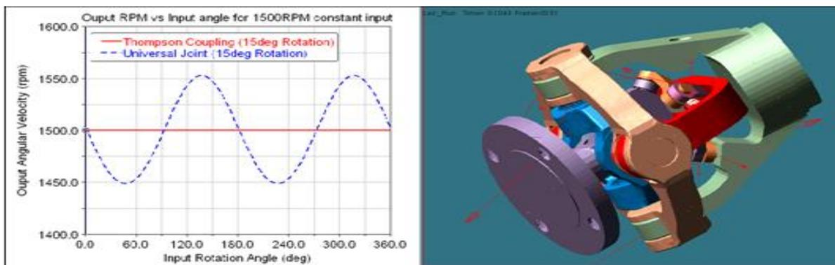
The graph above illustrates the difference in output motion of a universal joint (non-constant velocity) and a Thompson Coupling showing true constant velocity. The resultant non-constant velocity motion in traditional couplings produces shaft vibration and additional driveline forces causing increased wear and reliability issues for the power system.
