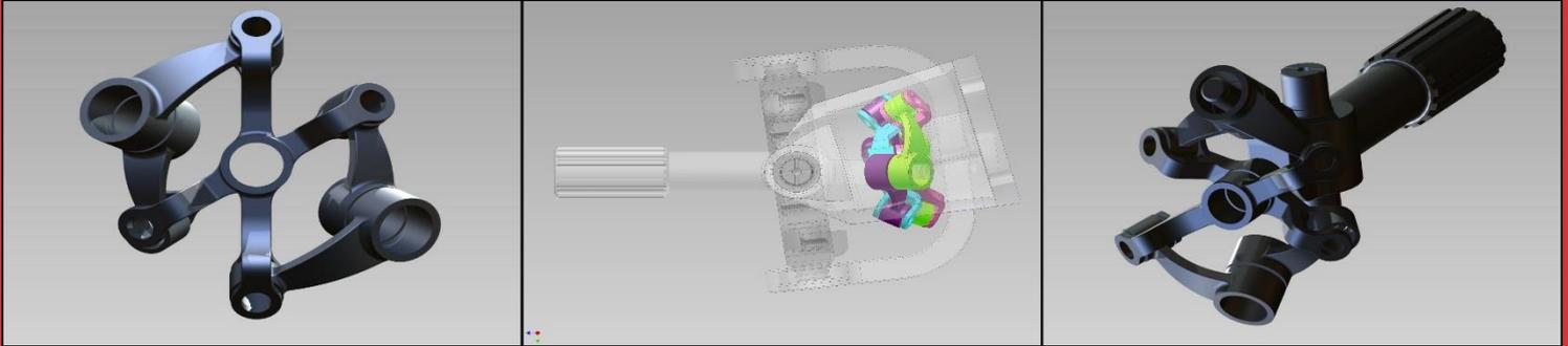
Graphic of the Thompson Coupling showing the internationally patented, spherical 4-bar linkage centring mechanism.
